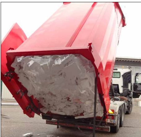
Compacted material does not fall out of the filling chamber.
